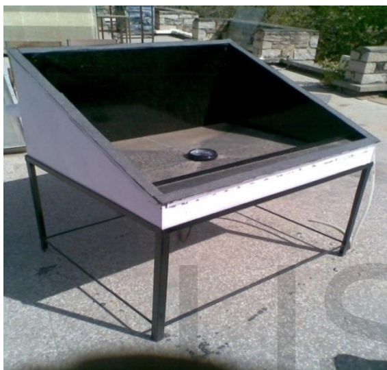
Fig. 1: Solar still walls painted with black epoxy paint from inside
