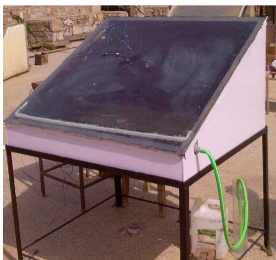
Fig. 2: Solar still with glass covering and outside walls painted white.
